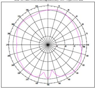
Far-field Power Distribution on Y-Z Plane(H-Plane of L3 Pol Sense) Gain=2.34dBi; Total Radiating Efficiency: 68.07% @2.50000 CHz
